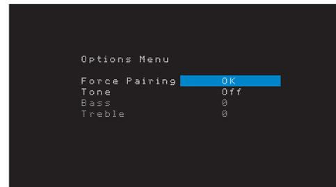
4. Select “Force Pairing > OK” and press the OK button. The AVR will enter the pairing mode.
