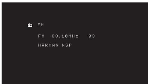
Use the Up/Down buttons or the Remote's Channel buttons to tune a station as displayed on the front panel and on-screen display.
