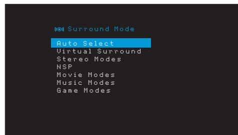
**Auto Select:** For digital programs, such as a movie recorded with a Dolby Digital or DTS soundtrack, the AVR will automatically use the soundtrack's native surround format. For two-channel analog and PCM programs, the AVR uses the HARMAN NSP mode.
