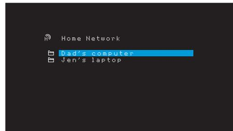
The screen will list by name all devices on the network that allow sharing. Use the Up/Down and OK buttons to browse the content stored in the device's media player library. Scroll to the desired item and press the OK button to select it. To return to the previous menu level (or to clear the menu from view from the top level), press the Back/Exit button.
